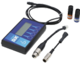
Dynamic programming unit For programming the Carony Go.
